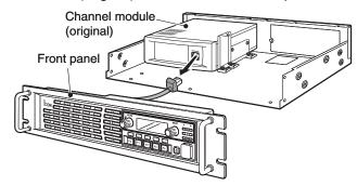
4 Remove 6 screws from the front panel, then remove the shielding plate and rubber seal.
